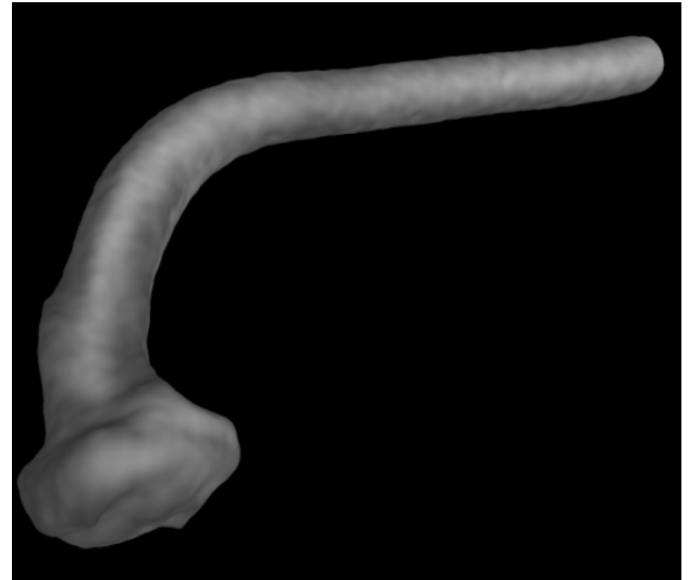
Figure 5– Close-up \mu CT of copper wirebond
