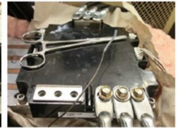
(b) thermocouple inserted through lid
